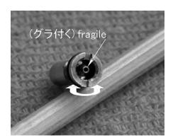
Please insert the other O-ring supplied to the back side gas inlet, as per photo shown below. To insert the O-ring properly, please use the tool supplied with the O-rings.
